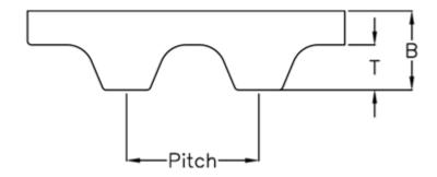
Height B mm= 2.2Height T mm= 1.2Length= 690Number of teeth= 138Pitch= 5Type $= PU \ 8 \ T5 \ 690$ Width= 8
